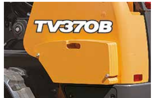
Additional Counterweight to increase ROC
