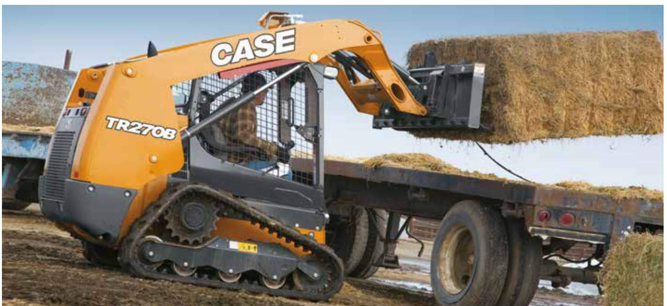
Additional Counterweight to increase ROC
