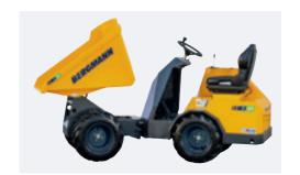
C801e – the little brother with a width of 980 mm and a payload of 950 kg
